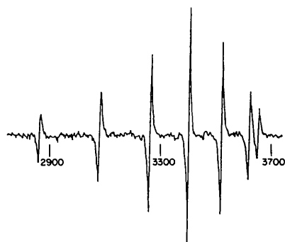
Fig. 2. EPR X-band spectrum of Gd^{3+} in europium bromate enneahydrate.
